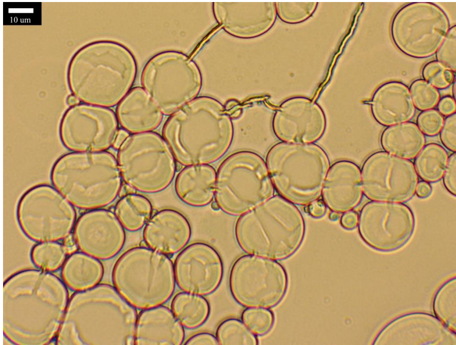
Figure 26: Micrograph of an emulsion containing 2 wt% total N20 silica and 0,1 CMC CTAB in the aqueous phase mixed with an equal volume of isopropyl myristate and let to dry in ambient air. The pH of the water phase was set only by the N20 particles. Aside from the long and narrow channels between a few droplets, a something like a solid film can be seen that shows marks of tearing on all droplets. The scale bar is 10 \mu\text{m} .
